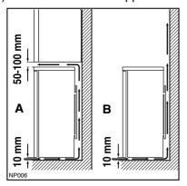
Do not obstruct the space underneath. The back of the cabinet may be placed close to the wall but must not touch it. DO NOT install in places with restricted ventilation. Adjust the level of the appliance by screwing out the adjustable foot, or feet, at the bottom of the cabinet using your fingers.
